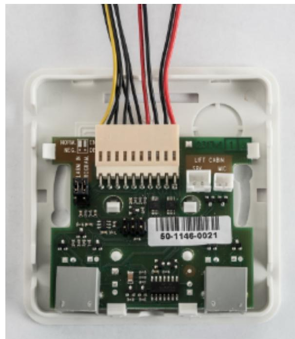
Connect the microphone and speaker from **2N® Lift1/ 2N® SingleTalk** in the point-switch. The speaker and microphone connectors are marked (SPK and MIC). Put the connectors on the jumpers in the switch. The configuration is the same as in **2N® Lift1/ 2N® SingleTalk** (also marked on the switch board). Pull the cables through the holes.
