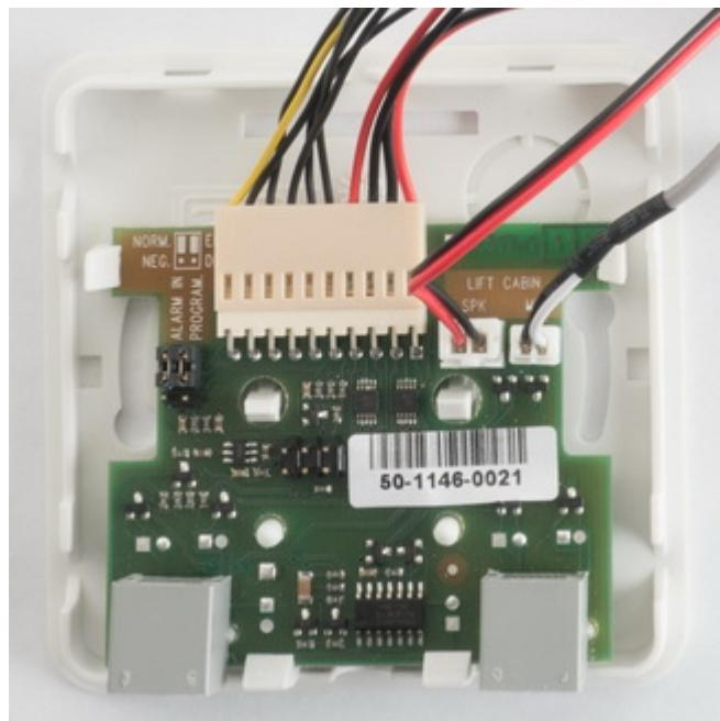
Break out cable holes in the switch upper cover. Then replace the cover. There are 2 RJ12 connectors on the point-switch side for audio unit connection. Interconnect the audio unit and the switch using the cable supplied.
